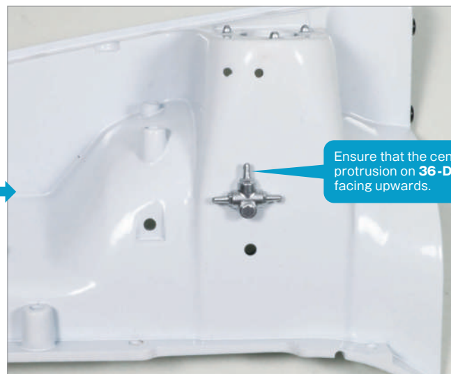
Turn 36-A over and fit the protrusion of the 36-D Front Brake Hose Connector into the hole on the inner side.
